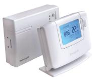
Intelligent room thermostat unit (accessory) with extension room thermostat (accessory) for the second circuit: Based on Outside Temperature Compensation (OTC). Water outlet target temperature is automatically recalculated taking into account the outdoor ambient temperature and the difference between the room setting temperature and the room actual temperature.
